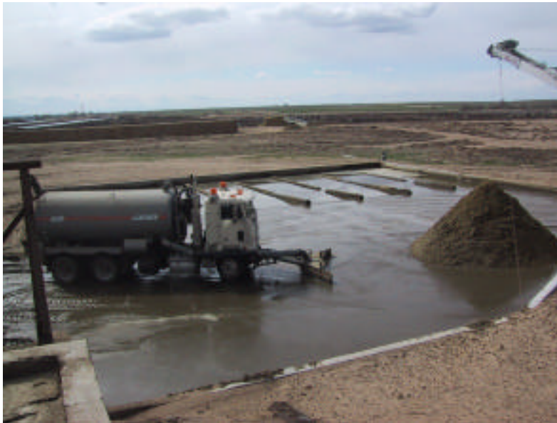
Vacuum Truck Collecting Manure Solids
