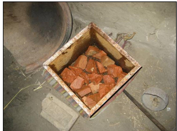
Brick chips and nails in a Kanchan™ filter
