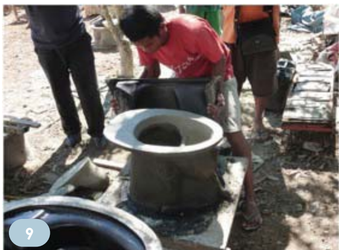
Pic 9/10: Construction of Urine Diversion Concrete Bowls (by WAND Foundation, Libertad)
