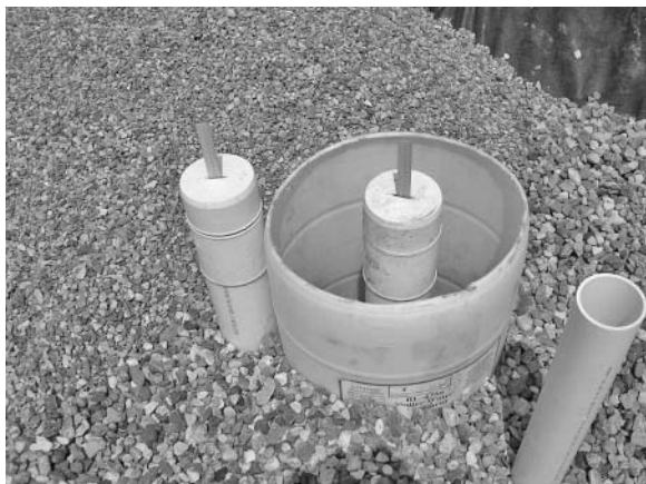
FIGURE 2.7 Water barrel apparatus to test liner leakage in a VF wetland, Diamond Lake Woods, Minnesota.
