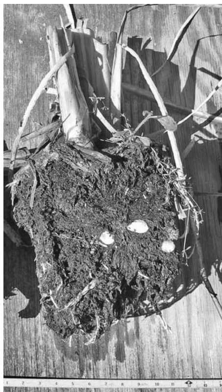
FIGURE 3.25 A section through the floating mat at the Houghton Lake, Michigan, treatment wetland. The cattail plants have been clipped about 15 cm above the mat, which is about 30 cm thick. Note the black sediment in the rhizome and root matrix.
