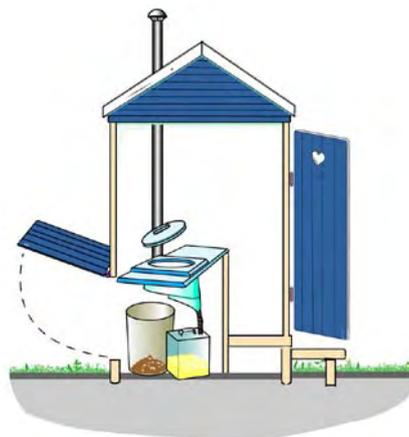
Figure 18. (right) Urine-diverting liner for outhouses. Picture by Palmcrantz and Co.
