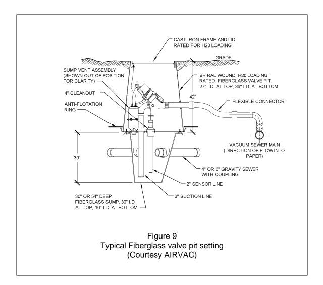
Up to four separate building sewers can be connected to one sump, each at 90 degrees to one another. However, this is rarely done as property lines considerations and other factors may render this impractical. By far, the most common valve pit sharing arrangement is for two adjacent houses to share a single valve pit (AIRVAC, 2005)
