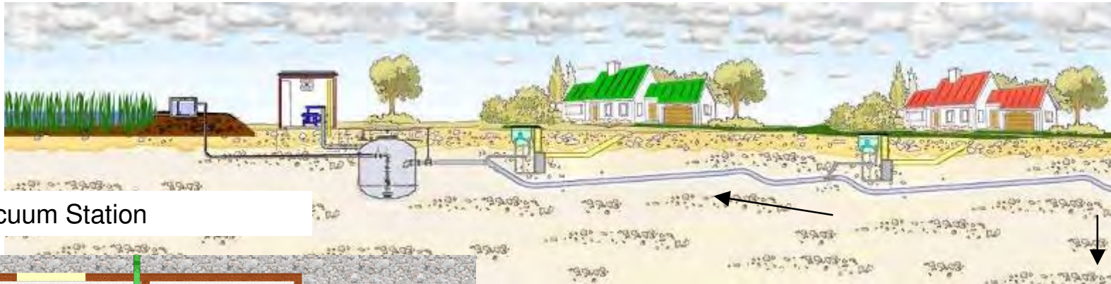
The Collection Chambers and Vacuum Collection Line
