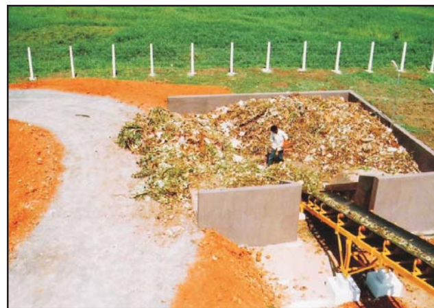
Vegetable Waste Loading on Belt Conveyor
