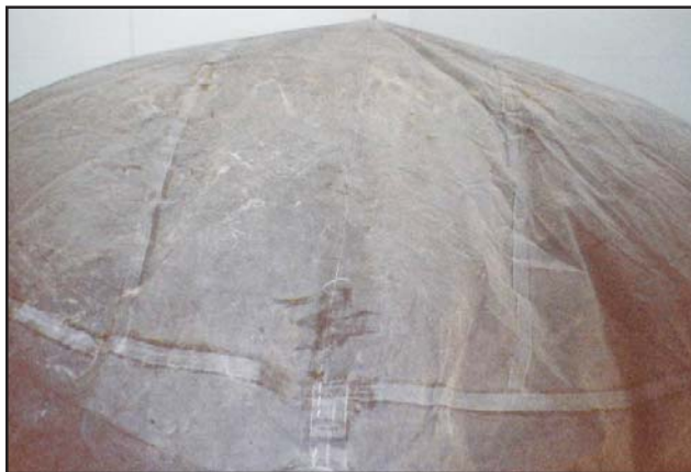
Dry Membrane Balloon Type Gas Holder
