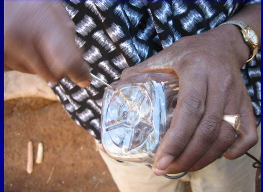
**Cut the bottom off about one third up. Make a hole in one corner of the base near the edge with a sharp nail or sharpened piece of wire.**
