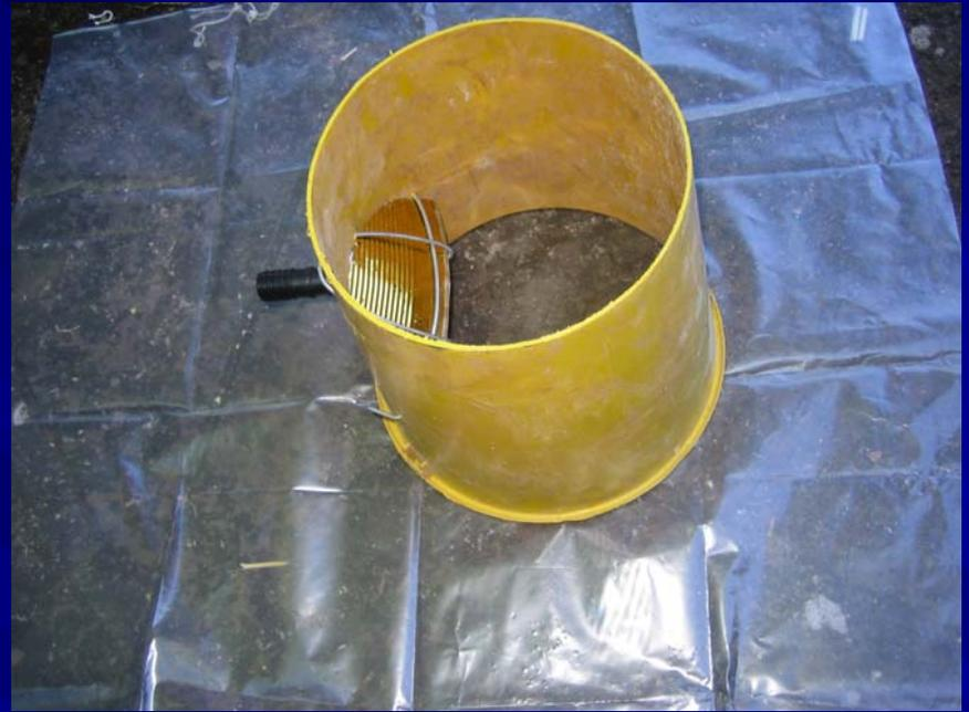
**One wire passes along the top of the tin sheet and through the bucket and is bent over at each end. This secures the tin well. Chewing gum is used to make a seal between the bucket and the tin sheet. The sheet can be replaced later if required. The wire is best galvanised so it lasts longer.**
