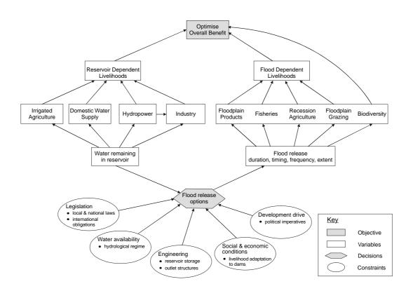
Figure 2.4.1 Flow chart showing the trade-off between using water for managed flood releases and for other purposes.
