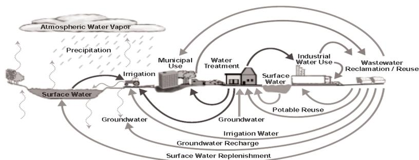
Figure 2. The role of engineered treatment, reclamation, and reuse facilities in the multiple uses of water through the hydrologic cycle (Asano and Levine, 1995).
