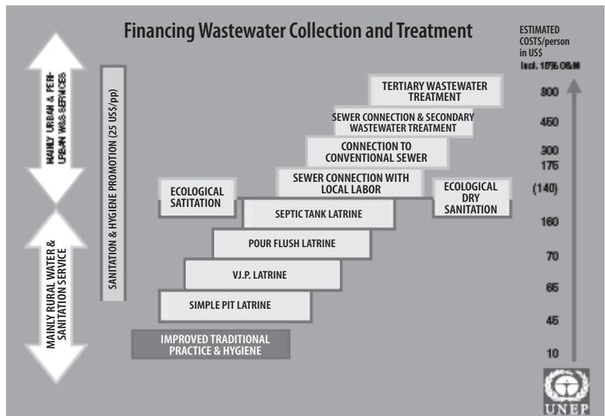
Figure 3. Costs of various services on the “sanitation ladder” (Water Supply and Sanitation for All, 4WWE, 2006).
