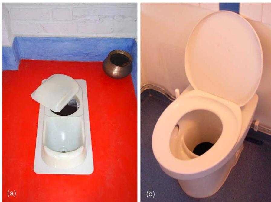
Fig. 5. (a) A urine-diverting dry squat toilet from India (photo: S.Vishwanath [www.rainwaterclub.org](http://www.rainwaterclub.org)); (b) a urine-diverting dry toilet from Sweden (photo: Dana Cordell).
