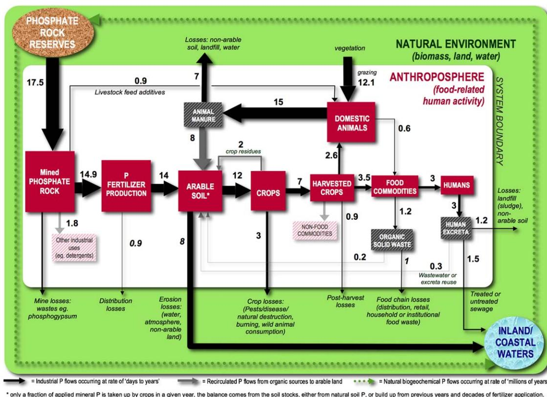
**Fig. 3.** Key phosphorus flows through the global food production and consumption system, indicating phosphorus usage, losses and recovery at each key stage of the process. Units are in Million Tonnes per year (Only significant flows are shown here, relevant to modern food production and consumption systems.). Calculations based on data in IFA (2006) and Smil (2000a,b).
