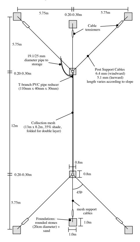
Figure 10-4 48m<sup>2</sup> FCU (Plan View)
