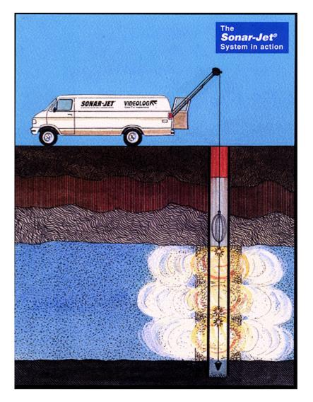
1. A mild "harmonic" (kinetic) frequency of shockwaves designed to gently loosen hardened mineral, bacterial or other type deposits, even heavy gypsum deposits almost impossible to attack chemically.
