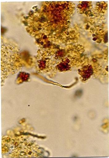
Bacterial iron can usually (but not always) be distinguishable visually from purely mineral iron incrustation by its soft, slimy feathery or appearance. and microscopically by the presence of bacterial structures and distinct mineral types. Under the microscope you can see the long, thin filaments or twisting stalks of various types which by microbiologists name the "iron bacteria".
