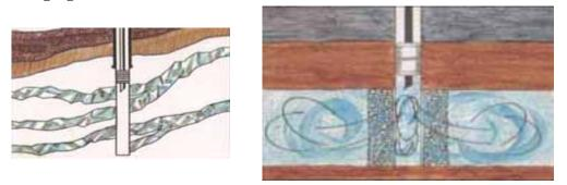
Step After treatment the well is mechanically developed using surge/airlift
