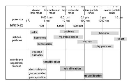
Fig. 1 – Membrane separation processes, pore sizes, molecular weight cut-off (MWCO) and examples of sizes of solutes and particles.
