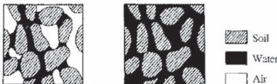
Figure 8. Unsaturated flow (left) gives better filtration and oxygenation of the water than saturated flow (right) (Jensson & Heistad, 2000).
