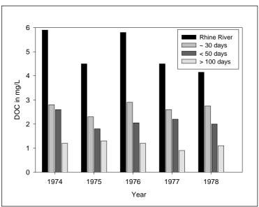
Fig. 8. DOC removal in bank filtration with different retention times.
